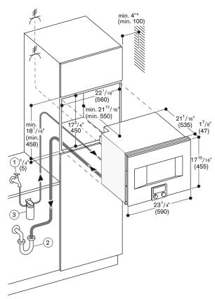
\* 8" (200) minimum when installed with handle.
