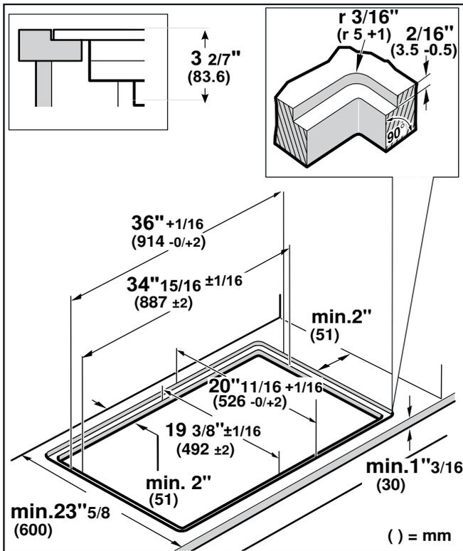
The appliance can be installed in the following temperature- and water-resistant countertops:
