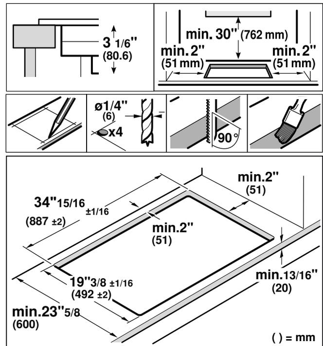
**Flush mounting:** Flush mounting into a countertop is possible.
