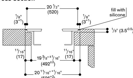
For installation with appliance cover or adjustment bar, observe the deeper notch and the slot width front and back.
