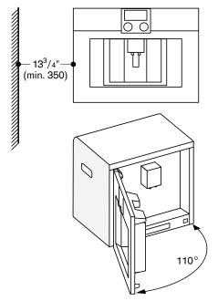
If using the 92° door hinge restrictor (spare part no. 00636455), the minimum distance to the wall is only  $3^{15}/_{16"}$  (100 mm).
