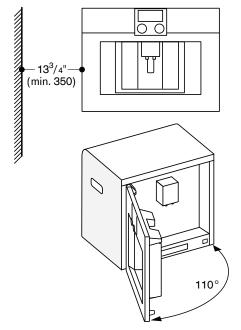
If using the 92  $^\circ$  door hinge restrictor (spare part no. 00636455), the minimum distance to the wall is only 3^{15}/16" (100 mm).
