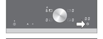
3 Use the twist knob to set the required duration between 1 and 90 minutes.
