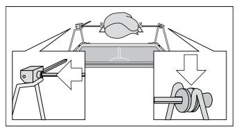
6 Insert the rotisserie spit in the lowest insertion level in the oven. The drive spindle must engage in the opening on the oven's rear wall.
