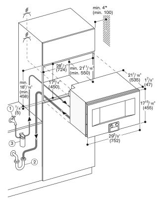
\* 8" (200) minimum when installed with handle.
