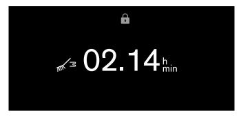
After the descaling program has finished, a signal sounds. The appliance door is unlocked. A message appears on the display.
