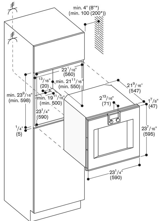
\* 8" (200) is minimum distance requirement in order to use pull-out system BA 016 105 and when installed with handle.
