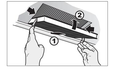
3 Insert the metal grease filters (see "Removing and inserting the metal grease filters").
