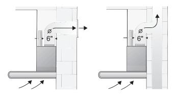
The exhaust air is discharged upwards through a ventilation shaft or directly through the outside wall into the open.
