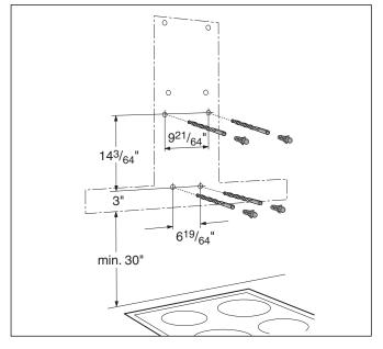
6 Attach the extractor hood. Adjust the height and align horizontally with the adjusting screws.
