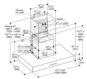
With the exhaust air duct cover AD 442 012 suitable
