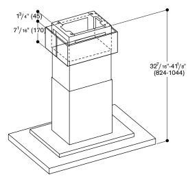
$^{\star}$  Suitable for ceiling heights of 8 ft (2.42 m) to 8.7 ft (2.64 m); Specifications refer to a distance from floor to lower chimney edge of 5.2 ft (1.60 m).
