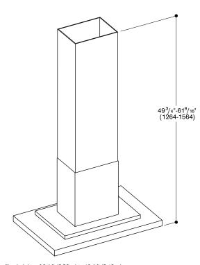
\* Suitable for ceiling heights of 9.4 ft (2.86 m) to 10.4 ft (3.16 m); Specifications refer to a distance from floor and lower chimney edge of 5.2 ft (1.60 m).
