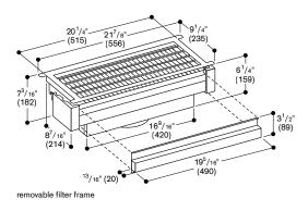
Numbers indicated inside parenthesis ( ) = mm Upper cabinet for AF visor hood with lowering frame AA 210 460/ AA 210 490
